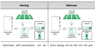
Optimized self-consumption will be achieved. ESS is used to store excess energy produced by PV system.
